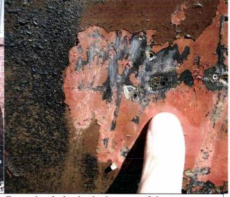
Corrosion holes in the bottom of the aboveground oil tank.
