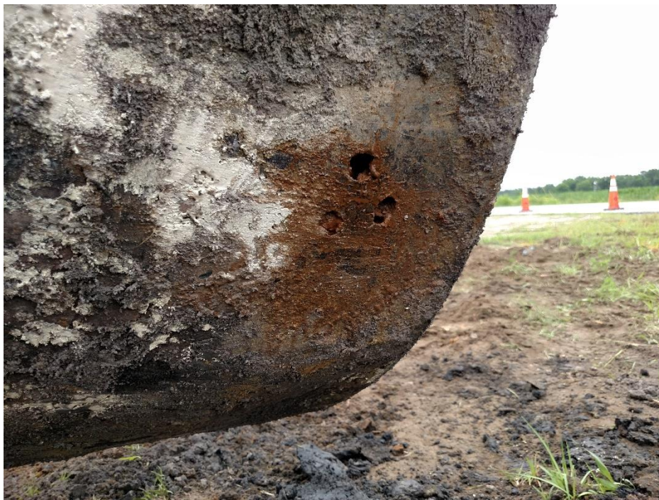
Photo #8: A view of the holes observed along the bottom of UST-2.
