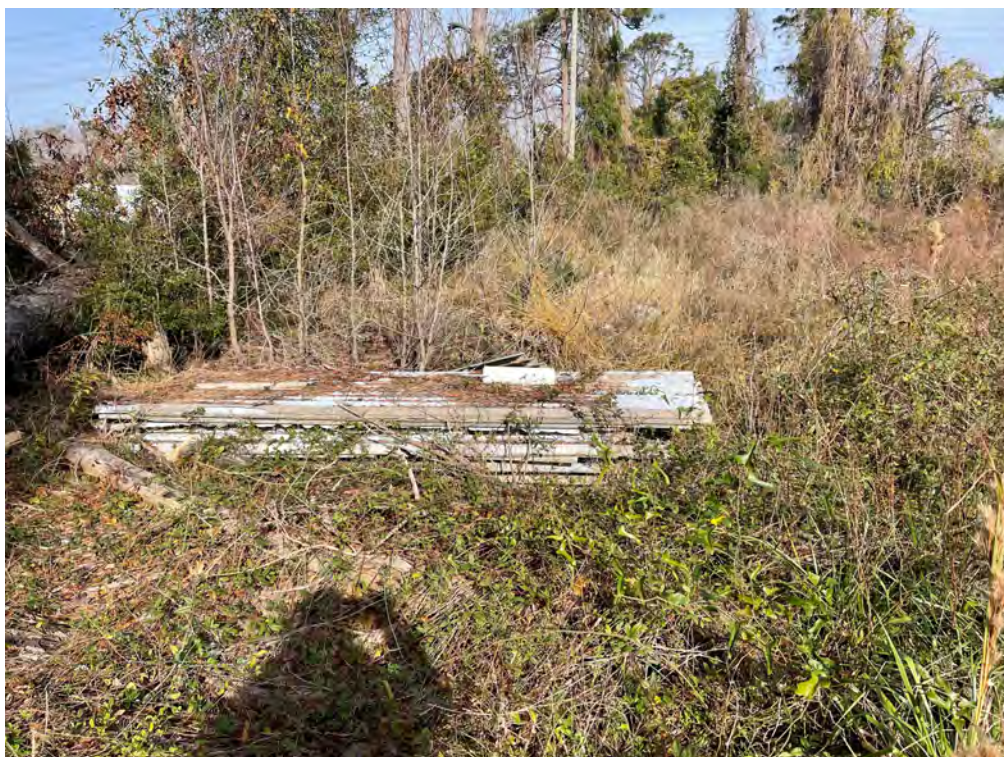
Photograph 14 – Suspect corrugated transite roofing sheets north of the on-site structure, along the western property boundary.
