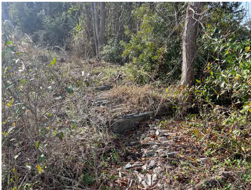
Photograph 15 – Suspect corrugated transite roofing sheets north of the on-site structure, along the western property boundary.
