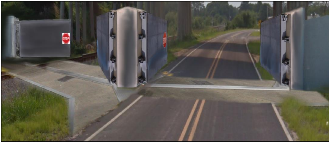
Figure 2-5: Conceptual View of VFW Road and CSX Railroad Underpass Floodgate
